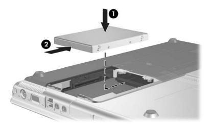
3. Align the tabs on the hard drive cover with the slots on the notebook • and press the hard drive cover down until it snaps into place •.
